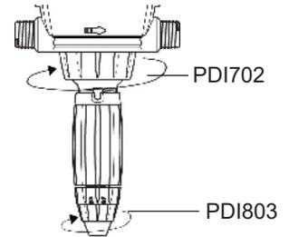
2. Unscrew check valve nut (PDI747) and pull out check valve assembly (PJDI118). It will come out in one piece. Discard.
