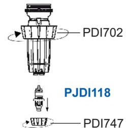
7. Push complete injection stem assembly in position at the bottom of the blue body, making sure desired scale is facing front of injector. Keys at the top of the black sleeve should slide into the slots at the bottom of the body. Slide injection stem nut (PDI702) up the sleeve and screw back on. Insert hose back onto the bottom of the check valve barb (PJDI118). Screw hose nut (PDI803) back on.
