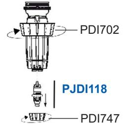
3. Unscrew locking nut (PDI746), remove "C" clamp (PDI751) by slightly spreading the opening and gently sliding it down over the threads. Unscrew adjusting sleeve (PPDI037). Holding the sleeve (PDI805), push up on the threaded part of the injection stem (PDI753) and slide it out of the sleeve from the top. Replace both sleeve and injection stem o-rings (JDI100 and JDI122).
